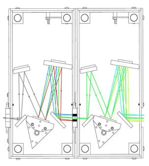
The 9072DA is made of 2 single monochromators in a additive mode: the dispersion of the second monochromator adds to that of the first one.
