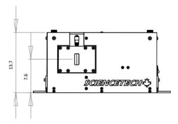
The dimension of 9072DA/DS is to double the single unit dimension of 9072. Sciencetech manufactures and integrates a full line of input and output couplings as well as a selection of beam line connections. Visit our website to look at all the possibilities:
